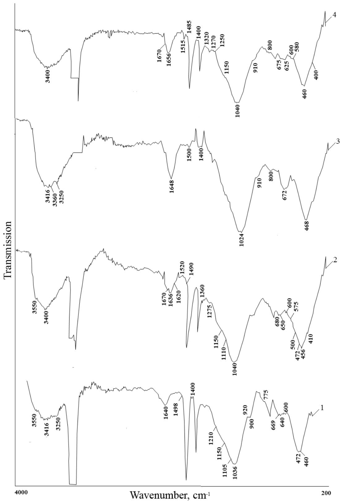
Fig. 3. IR-spectra of pure (1) and modified (2-4) powders
