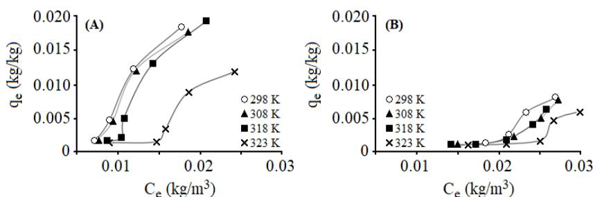
**Fig. 2.** Adsorption isotherms of DVB (a) and MMA-DVB (b). Initial oil concentration of  $0.03 \text{ kg/m}^3$ , temperature range of 298–323 K, contact time of 18000 s;  $q_e$  is the mass of oil adsorbed per mass of adsorbent in equilibrium, and  $C_e$  is the concentration of oil in water in equilibrium
