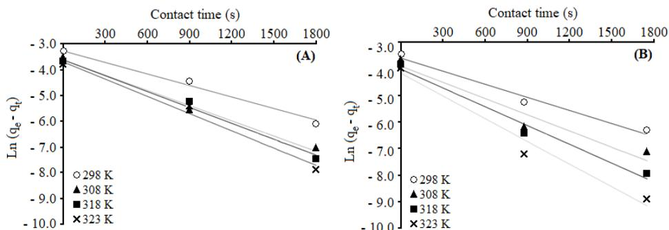
**Fig. 4.** Linearization of the pseudo-first-order adsorption kinetics of DVB (a) and MMA-DVB (b). Initial oil concentration of  $0.15 \text{ kg/m}^3$ , resin mass of  $3 \cdot 10^{-4} \text{ kg}$  and temperature range of 298–323 K
