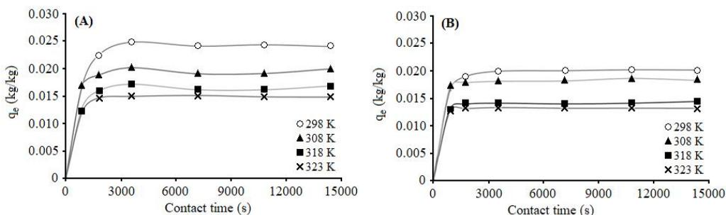
**Fig. 3.** Adsorption kinetics of DVB (a) and MMA-DVB (b). Initial oil concentration of  $0.15 \text{ kg/m}^3$ , resin mass of  $3 \cdot 10^{-4} \text{ kg}$  and temperature range of 298–323 K;  $q_e$  is the mass of oil adsorbed per adsorbent mass
