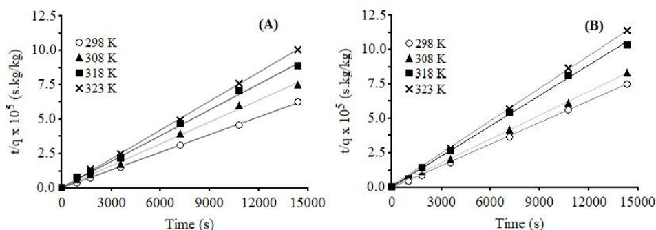
**Fig. 6.** Linearization of the pseudo-second-order adsorption kinetics of DVB (a) and MMA-DVB (b). Initial oil concentration of  $0.15 \text{ kg/m}^3$ , resin mass of  $3 \cdot 10^{-4} \text{ kg}$ , temperature range of 298–323 K, and contact time of 14400 s
