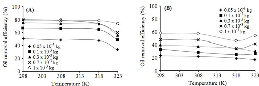
**Fig. 1.** Effect of temperature on the oil adsorption efficiency of DVB (a) and MMA-DVB (b), using resin masses of  $0.05 \cdot 10^{-3}$ ,  $0.1 \cdot 10^{-3}$ ,  $0.3 \cdot 10^{-3}$ ,  $0.7 \cdot 10^{-3}$  and  $1.0 \cdot 10^{-3}$  kg and oil concentration of  $0.03 \text{ kg/m}^3$
