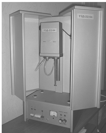
Fig. 1. The image of an ultrasonic generator UZDN-2T for combustion of inclusions of organic matters and disinfection of microorganisms in the ultrasonic field
