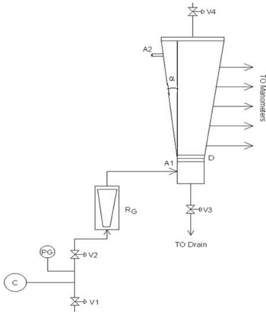
**Fig. 1.** Schematic diagram of experimental setup [2]:
