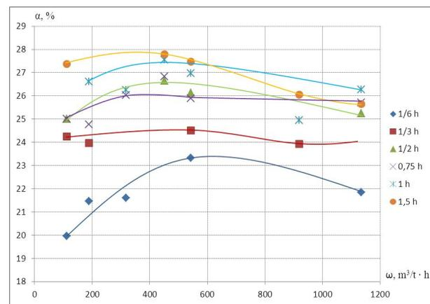
**Fig. 5.** Level of SO<sub>4</sub><sup>2-</sup> recovery from the solution and kainite into schoenite vs. intensity of air mixing
