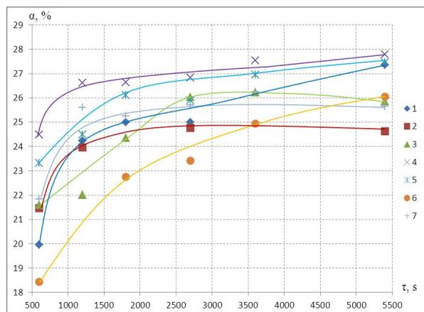
**Fig. 4.** Level of SO<sub>4</sub><sup>2-</sup> recovery from the solution and kainite into schoenite vs. process time under different intensity of air mixing (m<sup>3</sup>/t·h): 111.4 (1); 188.5 (2); 317.0 (3); 451.2 (4); 542.6 (5) and 919.6 (6)
