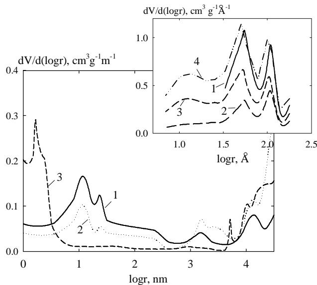
**Fig. 3.** Differential pore size distributions obtained by SCP method. Insertion: the distributions obtained by means of water vapour adsorption-desorption method. Ion-exchangers: pristine (1), modified with nanoparticles and their aggregates (2), containing only aggregates (3), the curve (4) corresponds to (3) data recalculated for the polymer
