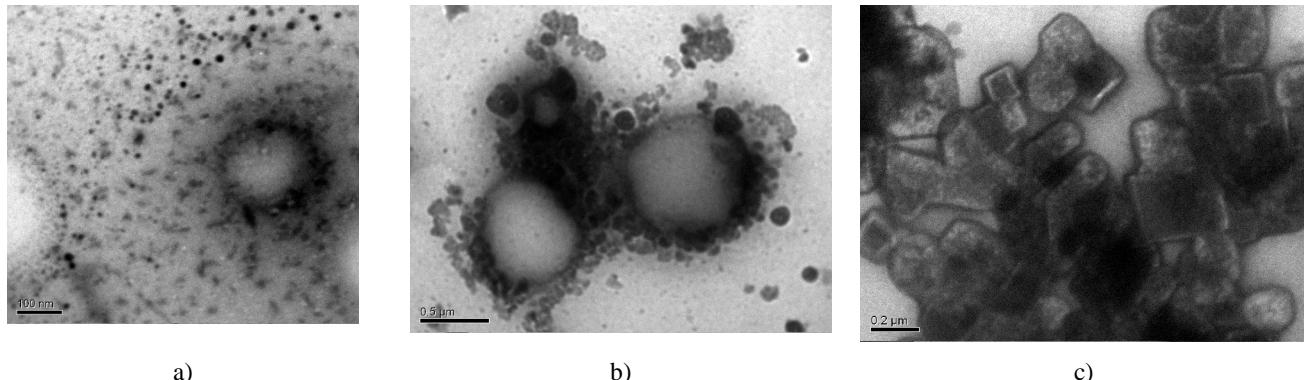
**Fig. 1.** TEM image of non-aggregated ZHP nanoparticles (a) and their aggregates in the polymer. ZHP was deposited from solution (a, b) and sol (c)
