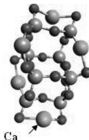
Fig. 3. The structure of zeolite cluster \text{Ze}(\text{SiO}_2)_{30} with 4 calcium ions
