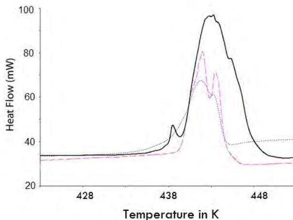
**Fig. 2.** DSC diagram for nifedrine: no UV exposure (—); 1 s exposure (....); 1.5 s exposure(---). Runs made at 20 K/min. Data were not normalized
