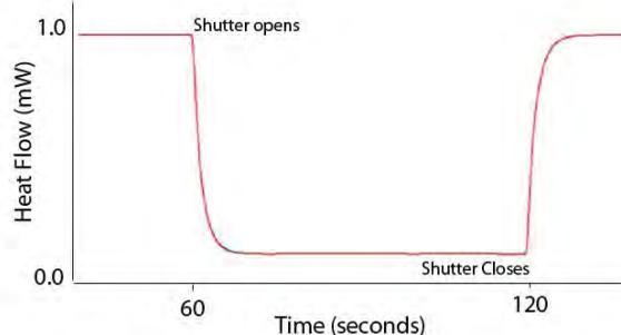
**Fig. 1.** Calculation of UV energy striking a graphite target for calibration within the DSC
