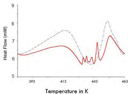
**Fig. 3.** DSC results for cetirizine: unexposed sample (---); 5 s exposure (—). Data were not normalized
