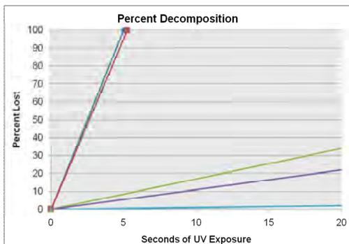
**Fig. 4.** Decomposition rates as a function of time of UV exposure. Lines from left to right: nifedrine, cetirizine, acetylsalicylic acid, pantoprazole and acetaminophen
