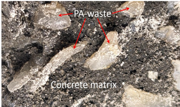
Fig. 14. SEM image of polyamide waste within the concrete structure
