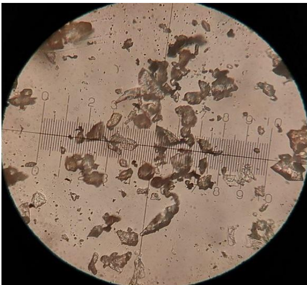
Fig. 5. 240x magnification (1 nicol): predominant fraction – the predominant size – fits the description of fine-grained sands
