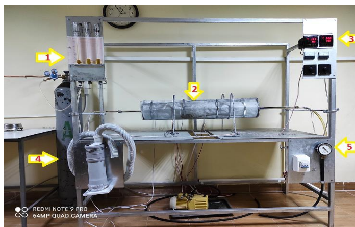
Fig. 1. Laboratory CVD unit for synthesis of MWCNT: 1 – gas treatment unit; 2 – two-section tubular reactor, blocks: 3 – temperature control unit; 4 – air supply; 5 – vacuum section
