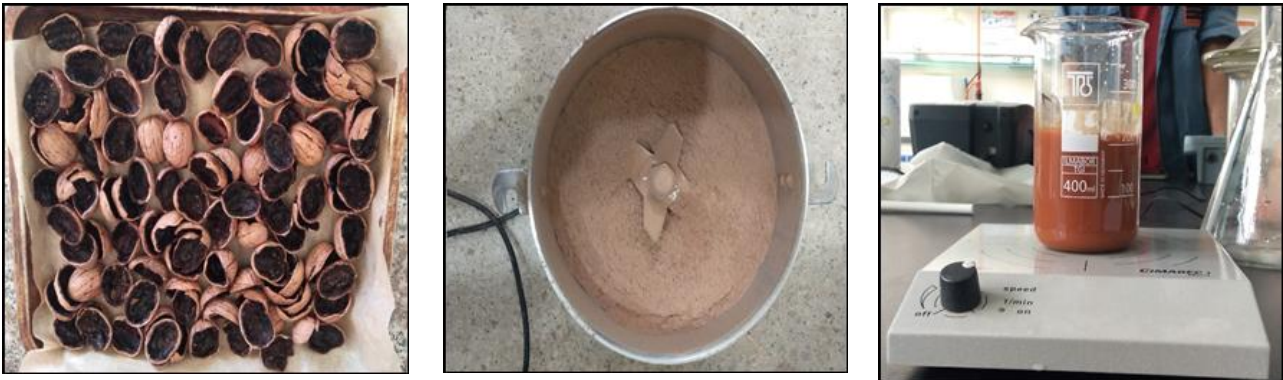
Fig. 2. Steps for preparing coagulant based on common walnut shells
