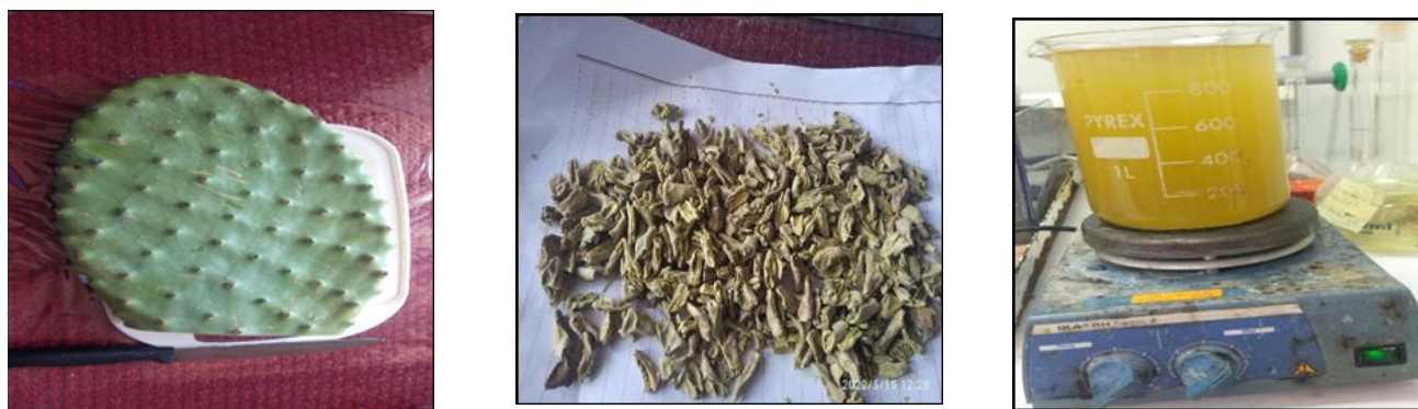
Fig. 4. Steps for preparing the coagulant based on Opuntia ficus-indica leaf powder
