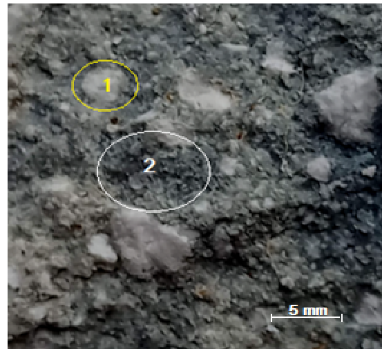
Fig. 2. Macrostructure of composite materials based on phosphogypsum: 1 – phosphogypsum flocs; 2 – cementing matrix
