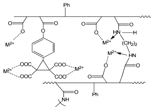
**Scheme 2.** Adsorption mechanism of resin for metal ions
