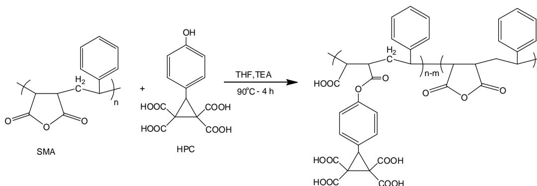
Scheme 1. Synthesis of SMA-HPC
