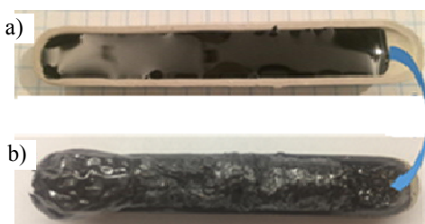
Fig. 2. Initial coal tar (a) and after heat treatment at 773 K (b)
