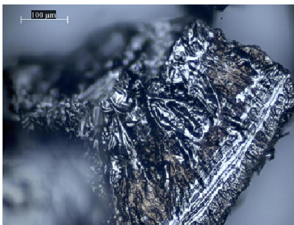
Fig. 4. Coal tar pitch after heat treatment at 773 K
