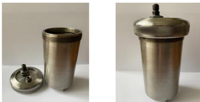
Fig. 3. Vessel for petroleum residues modification
