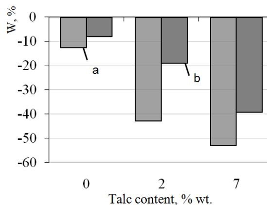
**Fig. 6.** Chemical resistance of PLA composites to the action of 5% NaOH depending on heat treatment (14<sup>th</sup> day): without heat treatment (a); with heat treatment (b)
