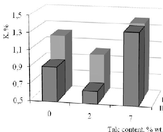
**Fig. 4.** Influence of talc content and heat treatment (I – without heat treatment; II – with heat treatment) on the swelling coefficient of PLA composites in 5%  $H_2SO_4$  solution
