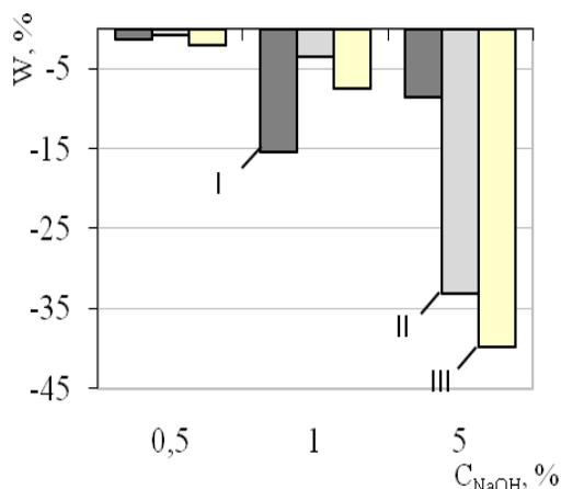
**Fig. 5.** Chemical resistance of PLA composites (10<sup>th</sup> day). Filler content (wt %): 0 (I); 2 (II) and 7 (III)
