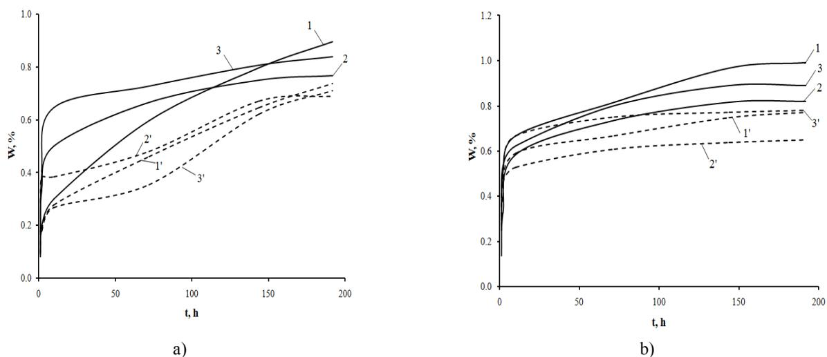
**Fig. 1.** Dependence of water absorption of polylactide materials on time at water temperature of 276 K (a) and 333 K (b). Talc content: 0 wt % (1, 1'); 2 wt % (2, 2'); 7 wt % (3, 3'). 1, 2, 3 – not heat-treated samples, 1', 2', 3' – heat-treated samples
